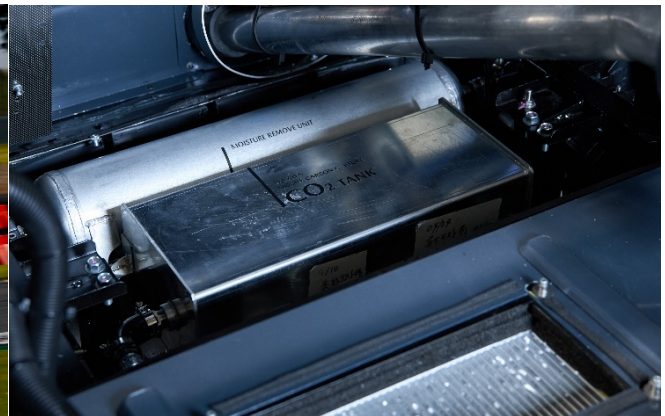
CO 2 capture system installed in the demonstration vehicle
